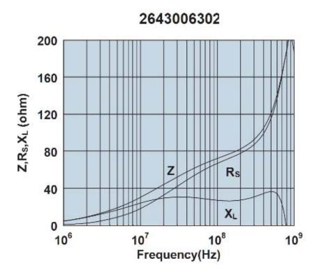
Impedance, reactance, and resistance vs. frequency.
