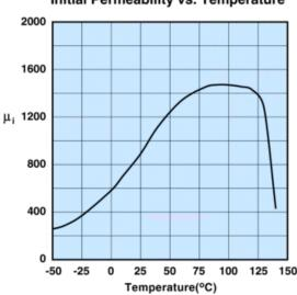
Measured on a 17/10/6mm toroid at 100kHz.
