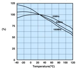
Measured on a 2643000301 using the HP4291A.
