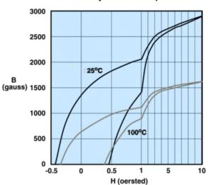
Measured on a 17/10/6mm toroid at 10kHz.
