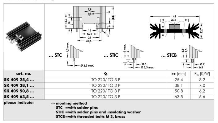
$\mathbf{P}$  = raised retaining stud,  $\mathbf{E}$  = mounting method special lengths and transistor drillings on request surface treatment: black anodised
