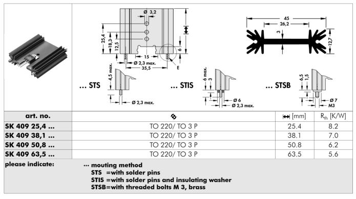
**E** = mounting method special lengths and transistor drillings on request surface treatment: black anodised
