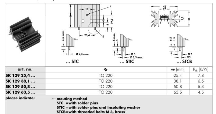
$\mathbf{P}$  = raised retaining stud,  $\mathbf{E}$  = mounting method special lengths and drillings on request surface treatment: black anodised
