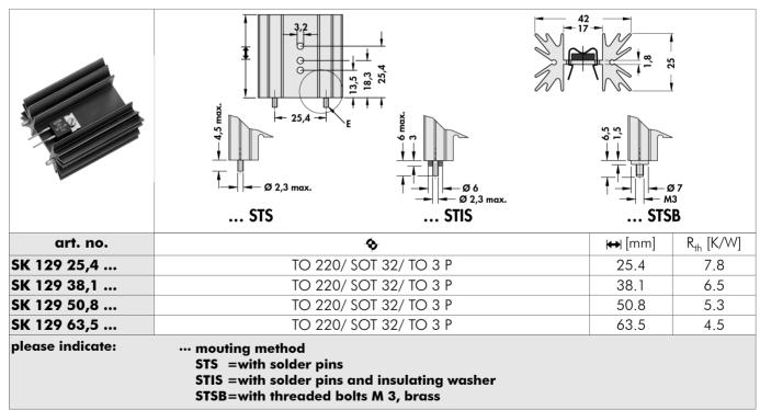
$\mathbf{P}=$  raised retaining stud,  $\mathbf{E}=$  mounting method special lengths and drillings on request surface treatment: black anodised
