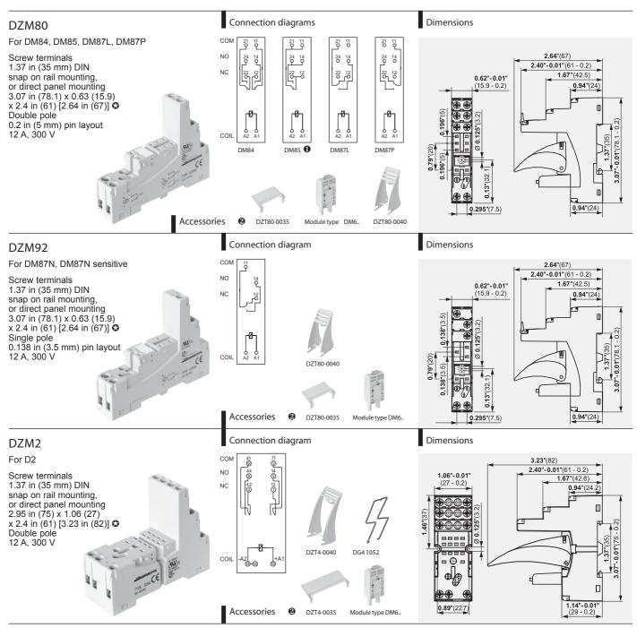
• For DM85: loads up to 12 A do not require bridging of common terminals. Loads above 12 A require
