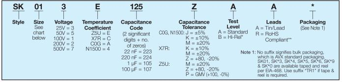
Note: Capacitors with X7R and Z5U dielectrics are not intended for applications across AC supply mains or AC line filtering with polarity reversal. Contact plant for recommendations.
