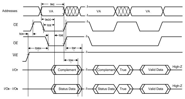
Note: VA = Valid Address. Illustation shows first status cycle after command sequence, last status read cycle, and array data read cycle.
