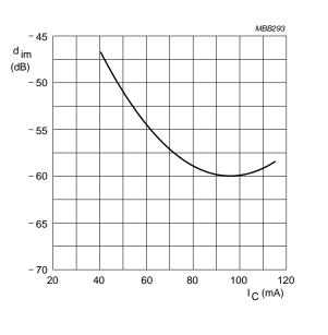
$V_{CE} = 10 \text{ V; } V_o = 850 \text{ mV; } T_{amb} = 25 \text{ °C; } \\ f_{(p+q-r)} = 793.25 \text{ MHz.}$
