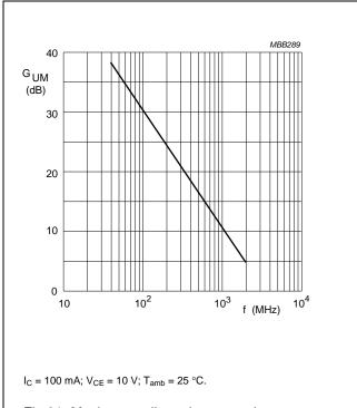
Fig.21 Maximum unilateral power gain as a function of frequency.
