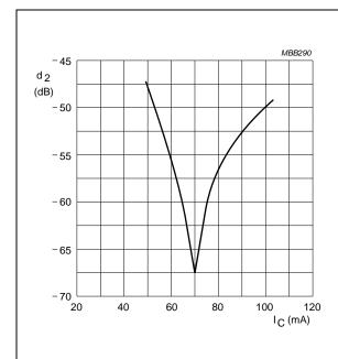
$V_{CE} = 10 \text{ V; } V_{o} = 50 \text{ dBmV; } T_{amb} = 25 \text{ °C} \\ f_{(p+q)} = 810 \text{ MHz.}$
