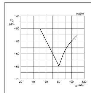
$V_{CE} = 10 \text{ V; } V_o = 50 \text{ dBmV; } T_{amb} = 25 \text{ °C; } \\ f_{(p+q)} = 450 \text{ MHz.}$
