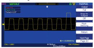
Generate user-defined pass/fail limits to quickly identify go/no go test results.
