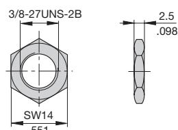
This is a metric design and millimeter dimensions take precedence ( $\frac{\text{mm}}{\text{inch}}$ )
