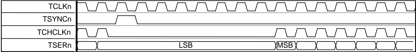
Figure 11-31. E1 Transmit-Side TCHCLKn Gapped Mode During Channel 1
