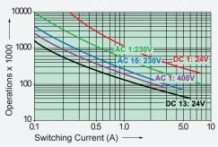
Maximal switching characteristics (DIN EN60947-5-1, Tab. C2)
