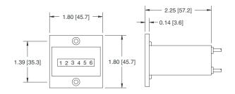
Mounting holes: For #5 flat head screw Panel cutout: 1.72" x 1.05" [43.7 x 26.7mm]
