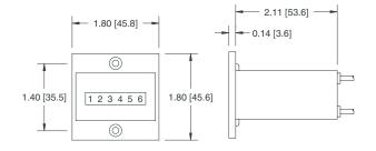
Panel cutout: 1.72" x 1.05" [43.7 x 26.7] Mounting holes: For #5 flat head screw
