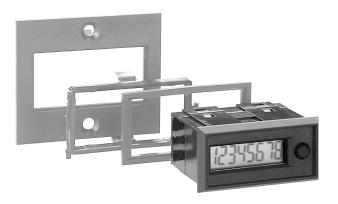
The Model 52 LCD 8-digit Miniature Electronic Counter offers a low cost general purpose miniature totalizer with a 10 year internal lithium battery. It is an economical replacement for electromechanical counters and is available for bi-directional or quadrature inputs. Front panel reset button can be enabled or disabled by a wiring connection or external contact closure. Easy snap in mount fits 0.94" x 1.89" [24 x 48mm] DIN panel cutout (0.98" x 1.97" [25 x 50mm] with adaptor).
