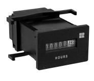
The Redington Model 711/731 provides a family of compact 7 figure, AC or DC Hour Meters. Models are available in the standard industry housings, 2-Hole rectangular, flush-round and flush-rectangular. DC Models are quartz controlled for high reliability and accuracy. A choice of two rectangular panel cutouts are offered 1.45" X 0.95" [36.8mm X 24.1mm] or 1.45" X 0.87" [36.8mm X 2.1mm]. The Round meter has a panel cutout of 1.99" [50.5mm].
