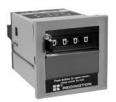
Designed for use in a wide variety of production, batching and packaging applications. These 4 or 6 figure electromechanical predetermining counters count down from a preset number and activate a SPDT switch. Convenient preset controls and built-in manual reset with guard are standard. A surge absorbing circuit protects against damage due to voltage spikes. Heavy duty bail mount secures counter in place.
