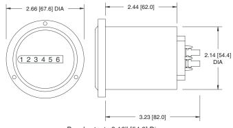
Panel cutout: 2.16" [54.9] Dia. Mounting holes: 0.125" [3.2] Dia. on 2.44" [62.0] B.C.
