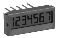
The Model 54 is a 7 or 8 digit LCD Totalizer with PCB mounting. Ideal for applications where PCB mounting, high reliability and long life are important. Units are 7 or 8 digits and come with their own lithium battery. Totalizers have two count speed ranges, 40cps or 150cps and are customer selectable.
