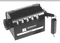
A 5 figure, rugged stroke counter, with right-hand shaft extension, operating lever and attached spring. Rated at 600 counts per minute, this heavyduty model is well suited for most industrial applications.
