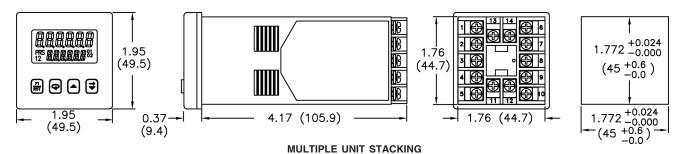
The Model 83 is designed for close spacing of multiple units. Units can be stacked either horizontally or vertically. For vertical stacking, install the panel latch with screws to the sides of the unit. For horizontal stacking, the panel latch screws should be at the top and bottom of the unit. The minimum spacing from center line to center line of the units is 1.96" (49.8 mm). This spacing is the same for vertical or horizontal stacking.
