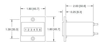
Mounting holes: For #5 flat head screw Panel cutout: 1.72" x 1.05" [43.7 x 26.7mm]
