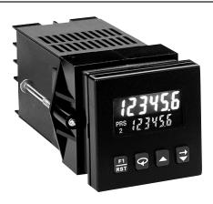
The Model 83 Timer is available in single or dual preset models. The 83 Timer features a 7 segment, 2 lines by 6-digit backlit LCD display. The main display line is red and shows the timer value. The smaller secondary display line is green and can be used to view the preset values or output time values.
