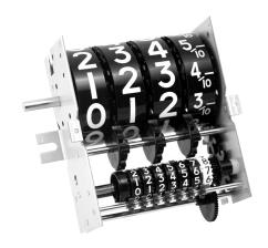
The Model 41 is a 3-figure or 4-figure mechanical register and is used to display gallons or liters output from a dispenser or pump. The large figure display can be reset with the rotary reset shaft. A smaller, non-reset, mechanical totalizer is also included to record total product dispensed.
