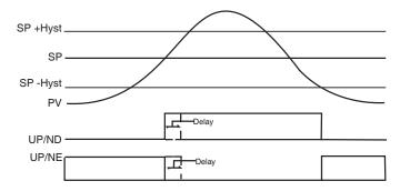
Output activates as input signal rises above setpoint (High Alarm)
