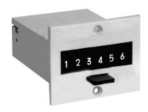
Economically priced 4 and 6 figure push-button reset, electromechanical counter designed for use where limited space is a factor and when reliability is critical. Rugged operating mechanisms require no lubrication or maintenance. Compact size and minimum space requirements make the Model 49 ideally suited for use in control panels, business machines, and test equipment.
