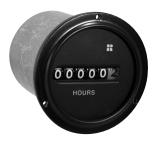
A 5 figure (reset) or 6 figure (non-reset), AC hour meter encased in a rugged steel housing and designed to mil-spec environmental requirements. The non-reset models are completely sealed, and meet NEMA 4 standards. Reset models are available, as are both wire lead and terminal block versions.
