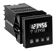
The 83 Counter features a 7 segment, 2 lines by 6-digit backlit LCD display. The main display line is red and shows the count value or the batch/ total value when preset 3 or output 3 is viewed in the secondary display. The smaller secondary display line is green and can be used to view the prescaler value, preset values, output count values or batch/total count values (batch model only).
