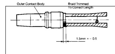
Slide the outer contact body over the intermediate contact assembly and ferrule until approximately 1.5 mm of the ferrule is visible. Trim off the excess braid using the rear of the outer contact body as a guide. Ensure that there are no loose braid clippings at the rear of the ferrule.
