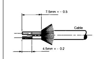
Remove outer sheath of cable to 7.5mm comb out all braids evenly and fold back. Remove cable fillers from stripped length. Strip the centre contact conductor to 4.5mm. Note: It is recommended that both intermediate and centre contact conductors are scored at the correct stripping length. The intermediate conductor insulation should not be removed until the centre contact has been crimped.
