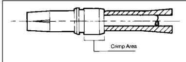
Place the outer contact body into the hexagonal cavity of the crimp jaws (294GB-5026-1). Slide the intermediate contact assembly and ferrule fully into the outer body using the insertion tool. The rear of the ferrule should be -0.5 or  $\pm$  0.5 mm to the rear of the outer contact body when fully inserted. Complete the hexagonal crimp.
