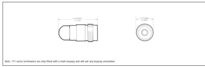
XX Refers to the terminator impedance value. This value can be selected according to the characteristic impedance of the data bus transmission line or to simulate the RT internal impedance. Amphenol standard terminators come fitted with two impedance values.
