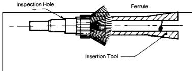
Slide the ferrule forward under the braid to trap the braid against the rear of the intermediate contact insulator, for all succeeding operations keep the ferrule firmly against the rear of the insulator using insertion tool (294GB-5028).
