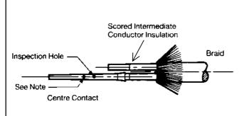
Crimp centre contact (Pin or Socket) on to the stripped wire using tool M22520/2-01 and crimp positioner 294GB-5027-1 (setting No. 4 for 24AWG) butting rear end of contact to wire insulation. The conductor end should be visible in the inspection hole. Note: A second hole is permissible in the socket contact for manufacturing purposes. It is not required to be on the same centre line as the inspection hole.
