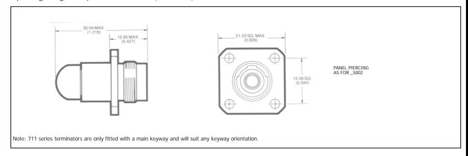
In Line Receptacle Terminator (3K $\Omega\pm5\%$ ) - 5028 - XX/C2846-/
