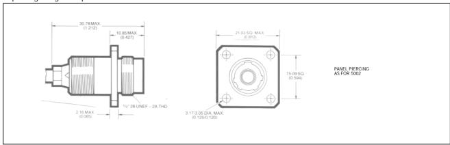
Single Hole Mtg. Receptacle with bulkhead seal and P.C. Termination Contacts-711-5038-
