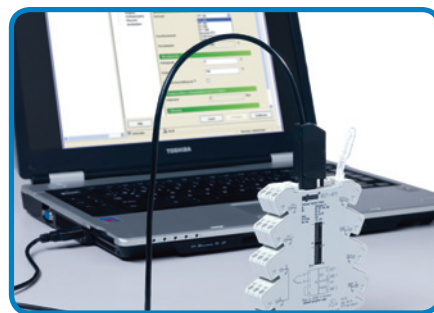
Configuration of the Transducers with WAGO-USB-Service-Cable 750-923
