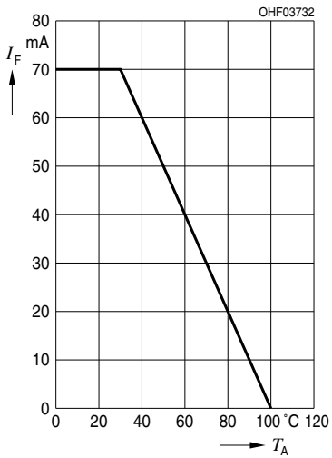
Max. Permissible Forward Current Max. zulässiger Durchlassstrom I_{F, \text{max}} = f(T_A), R_{thJA} = 500 \text{ K/W}
