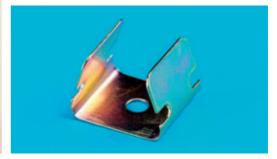
It is a requirement of BS5839 Part 1 that surface mounted Fire Performance cables must be secured using metallic fixings that can withstand the same temperatures and vibration as the Fire Performance cables.
