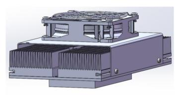
assembly from where heat is pumped by Peltier thermoelectric modules and dissipated to the environment through the use of bespoke heat sinks and highly efficient DC fans at the hot side of the assemblies. The thermoelectric modules, whose reliability and maintenance-free operation has been proven by the years, are carefully selected for each assembly to ensure the best cooling performance and minimise power consumption.
