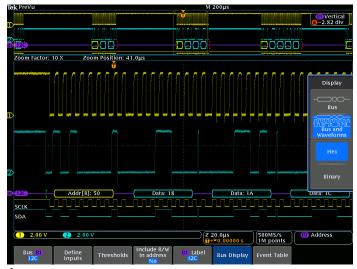
$\ensuremath{^{12}\text{C}}$  bus setup, showing selection of bus display modes.
