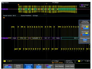
MIL-STD-1553 bus setup, showing threshold entry fields.
