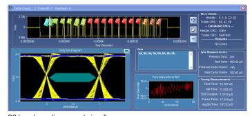
PC-based, eye-diagram analysis software builds an eye-diagram from the entire acquisition and plots it against TP1 mask called out by the FlexRay standard, available with MSO/DPO4000B and MDO4000B instruments.
