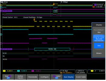
Simultaneously display the bus and digital waveforms. Digital waveforms show how the bus translates the individual signals based on the threshold settings (useful for making analog channels look like just 1s and 0s).
