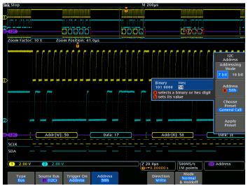
Triggering on a specific address value on the I<sup>2</sup>C bus.
