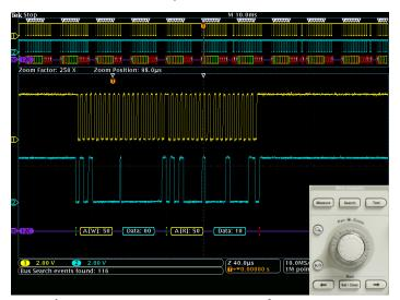
Search – I<sup>2</sup>C decode showing results from a Wave Inspector<sup>®</sup> search for Address value 50. Wave Inspector<sup>®</sup> controls provide unprecedented efficiency in viewing and navigating waveform data.
