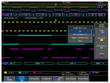
$\ensuremath{\text{I}}^2\ensuremath{\text{S}}$  bus setup, showing input configuration options for  $\ensuremath{\text{I}}^2\ensuremath{\text{S}}$  bus.
