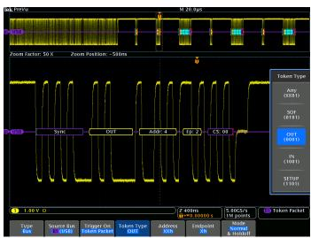
Triggering on a specific PID on a USB FS bus.
