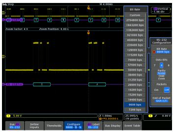
RS-232 bus setup, showing bit rate options for RS-232 bus.
