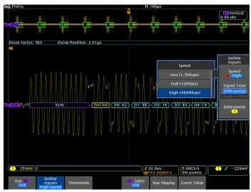
High-speed USB decoded display, automatically displaying bus content.
