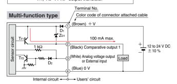
Symbols ... D<sub>1</sub>, D<sub>2</sub>: Reverse supply polarity protection diode Z<sub>D1</sub>: Surge absorption zener diode
