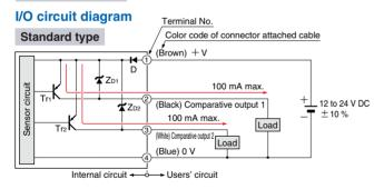
Symbols ... D : Reverse supply polarity protection diode  $Z_{D1}, Z_{D2}$ : Surge absorption zener diode  $T_{r1}, T_{r2}$ : PNP output transistor
