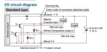
Symbols ... D : Reverse supply polarity protection diode  $Z_{D1}, Z_{D2}$ : Surge absorption zener diode  $T_{r1}, T_{r2}$ : NPN output transistor
