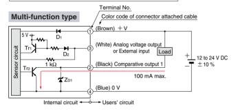
Symbols ... D<sub>1</sub>, D<sub>2</sub>: Reverse supply polarity protection diode
