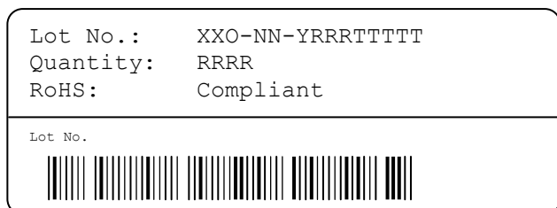
Figure 20: First label on reel: XX = Sensor Type (21 for SHT21), O = Output mode (D = Digital, P = PWM, S = SDM), NN = product revision no., Y = last digit of year, RRR = number of sensors on reel divided by 10 (200 for 2000 units), TTTT = Traceability Code.
