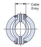
Note: Screw orientation shown is for non-self-locking configuration. Screws on self-locking configurations are on the same side/face of the clamp.
