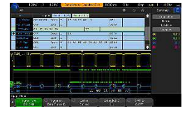
Figure 19: Multi-bus time aligned decode
