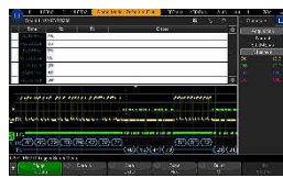
Figure 16: RS232 decode and trigger
