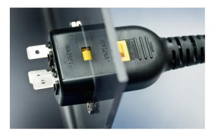
The lock is released by pressing a finger on the disengaging lever. This lever is easily identified due to its bright yellow color, a feature that also distinguishes this scheme from conventional pluggable power supply systems. The extraction force is at least 200 N.
