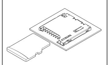
This is the connector for micro-SD card connector in which mounting height of 1.4mm maximum is kept and push-push mechanism is adopted.
