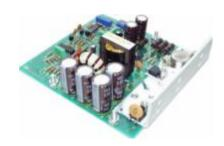
Description: Versatile switching regulator with a single adjustable stabilized output from a DC Source.
