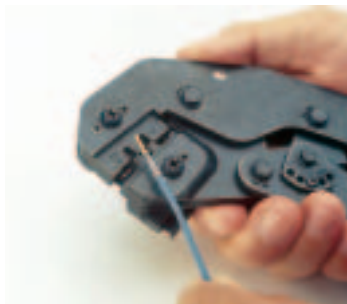
7. The result will be a perfect termination.
