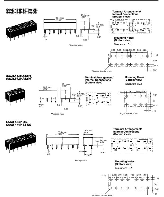
**ALL DIMENSIONS SHOWN ARE IN MILLIMETERS.**To convert millimeters into inches, multiply by 0.03937. To convert grams into ounces, multiply by 0.03527.
