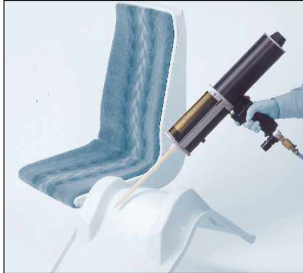
Bonding a seat cover to the ABS moulding 3M Scotch-Weld DP 190
