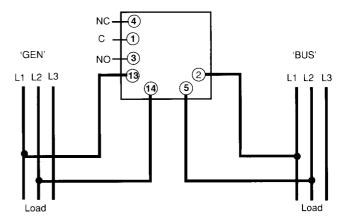
The 244-14D/H and 077-14D operate in the same way as the 244-14L and 077-14L Synchro check relays with the addition of a dead bus option. This optional feature enables the relay to energise with a GEN supply only thus allowing the generator to power the BUS during a supply failure.
