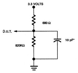
\* INCLUDING SCOPE AND JIG CAPACITANCE
