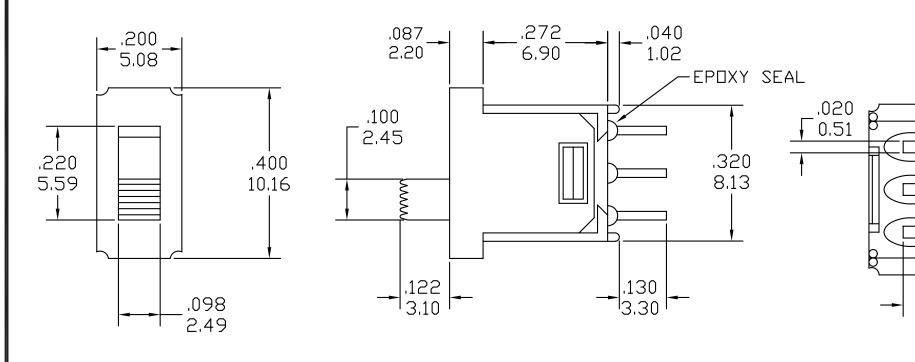
Rated current : 3A, 120VAC/ 1.5A, 250VACContact Resistance:  $10m\Omega$  MAX (initial)
