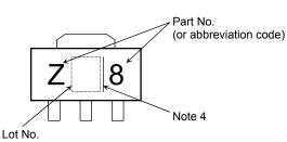
Note 4: A line to the right of a Lot No. identifies the indication of product Labels. Without a line: [[Pb]]/INCLUDES > MCV With a line: [[G]]/RoHS COMPATIBLE or [[G]]/RoHS [[Pb]]
