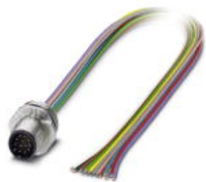
Sensor/actuator flush-type plug, 12-pos., M12 SPEEDCON, front/screw mounting with M16 thread, with 0.5 m PVC litz wire, 12 x 0.14 mm 2
