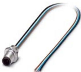
Sensor/actuator flush-type plug, 4-pos., M5, prewall/screw mounting, with M5 thread, with 0.5 m TPE litz wire, 4 x 0.14 mm 2
