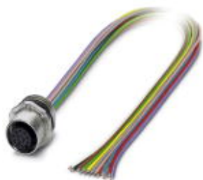
Sensor/actuator flush-type socket, 12-pos., stainless steel, front/screw mounting with M16 thread, with 0.5 m PVC litz wire, 12 x 0.14 mm 2
