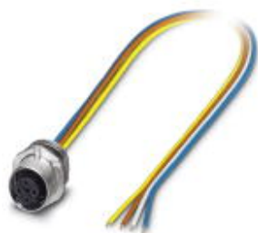
Bus system flush-type socket, PROFINET, 4-pos., M12-SPEEDCON, D-coded, front/screw mounting with M16 thread, with 0.5 m TPE litz wire, 4 x 0.34 mm 2
