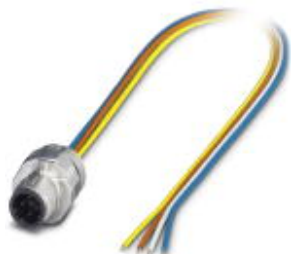
Bus system flat-type plug, 4-position, PlugLink:straightLink:M12-SPEEDCON, D-coded, Front mounting, can be positioned, M16 x 1.5, Individual wires, Cable length: 0.5 m
