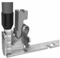
Principle of push-in connection
