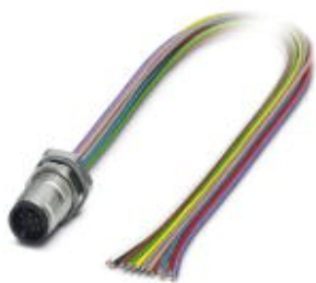
Sensor/actuator flush-type plug, 12-pos., M12 SPEEDCON, rear/screw mounting with M12 thread, with 0.5 m halogen-free TPE litz wire, 12 x 0.14 mm 2
