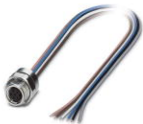
Sensor/actuator flush-type socket, 6-pos., M8, rear/screw mounting with M12 thread, with 0.5 m TPE litz wire, 6 x 0.14 mm 2
