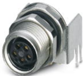
Sensor/actuator flush-type connector, socket, 5-pos., DeviceNet™, M8, rear/screw mounting with M10 fastening thread, with angled solder connection
