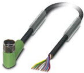
Sensor/Actuator cable, 8-position, PUR halogen-free, black RAL 9005, free cable end, on Socket angled M8, Cable length: 5 m
