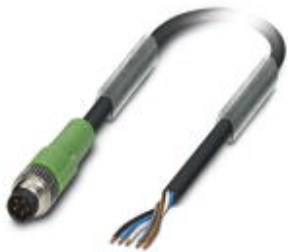
Sensor/Actuator cable, 5-position, PUR, black-gray RAL 7021, Plug straight M8, B-coded, on free cable end, Cable length: 3 m
