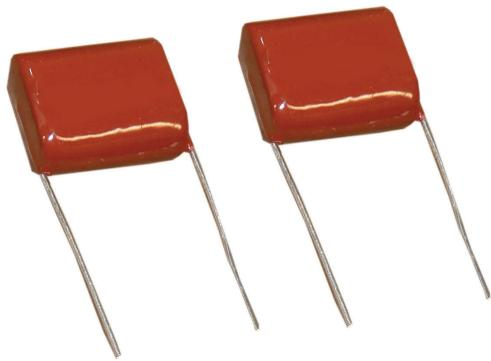
Type DPFF radial leaded polypropylene film/foil capacitors feature single and series section construction. Part numbers with the "S" suffix have extended aluminum foil with a floating metallized film. Excellent temperature stability to 105 °C and low loss characteristics, make Type DPFF ideal for high AC current and pulse applications.
