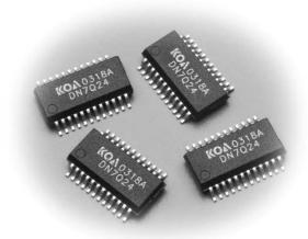
This diode network is designed to provide eighteen channels for active termination of high-speed data signals to eliminate signal undershoot and overshoot. The network has the added benefit of acting to suppress any ESD voltage events by shunting the energy to ground assuring maximum reliability of electronic systems in the field. Trigger levels are defined by the positive and negative bias levels set by the user.
