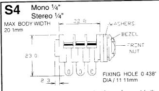
Mounting is effected by screwing the chrome facia nut (with plastic bezel) into a threaded plastic bush which protrudes from the body. Coloured bezels may be used. Contacts are NIAG alloy. The back of the socket is closed to prevent access through the socket. Ordering code as for S2. When ordering a mono type specify centre contact as 'N' e.g. S4/SNS/BLK. PC mounting versions - See below.
