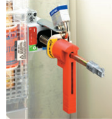
Door open: A strong metallic padlock kit allows up to three padlocks. The padlocking means is easily accessible, when locked closing of the disconnect is not possible.
