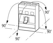
With residual-current release NZM1, N(S)1: Vertical and 90° in all directions
