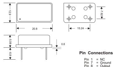
Pin 7 = Ground Pin 8 = Output Pin 14 = +V DC
