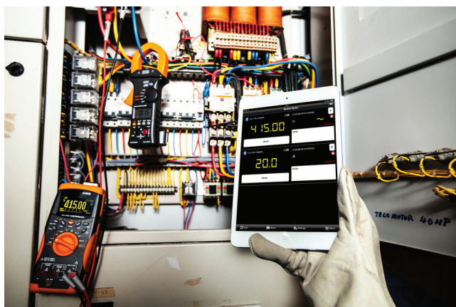
Figure 2. Monitoring handheld multimeter and clamp meter readings remotely via iOS/Android based smart devices
