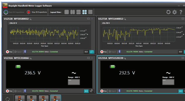
Figure 13. View up to 10 handheld meters readings or trends with Keysight Handheld Meter Logger software
